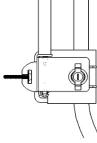
Now Attach your equipment carrier to the Action rack by inserting a carriage bolt with track washer into track and fastening equipment carrier. Some carriers may require some modifications
