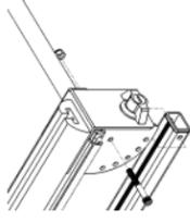
Set ActionRack Assembly on Load Bars. Line pivot holes on pivot, with the holes you drilled in loading bars.
