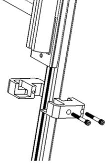
Place Latching Blocks around Load Bars pull tight until they seat on the slide. Inserts bolts and tighten till snug, using Allen Wrench supplied. Do not fully tighten, yet.
