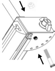
Place an adjustment bolt in each pivot adjustment hole, use the middle holes for now. Do not over tighten. Nut should be flush with threaded end of bolt. Operate rack several times to be sure everything is properly aligned.
