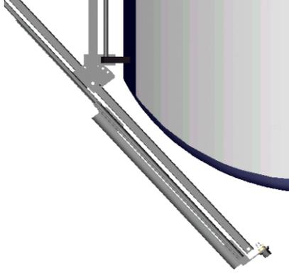
Now you may reposition the load position bolts on the pivoting unit to desired loading (down) position. **DO NOT** have the Action Rack too close to the side of your vehicle, as the weight of equipment could flex the load bars and cause the ActionRack to damage the side of your vehicle.
