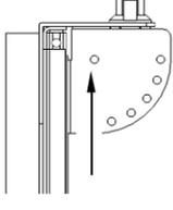
Identify the pivot hole on the pivot bracket located on the ActionRack Assembly.
