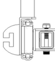
Slide pivot bolt through Pivot bracket holes and through load bar holes.
