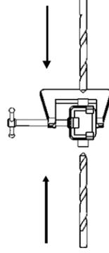
**Drill through one wall of loading bar at a time. DO NOT attempt to drill straight through. When finished drilling remove clamp and jig.**
