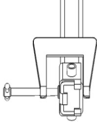
**Slide Drill Jig onto the end of Loading Bar till it stops. Secure with Clamp (Optional but recommended).**
