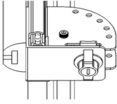
Turn the lock clockwise to the locked position it should turn freely and be in the center of the locking slot. If not, loosen latching block bolts and move the latching block, then snug bolts and repeat above steps until slides, latching blocks, and locks are in sync. Tighten latching blocks.
